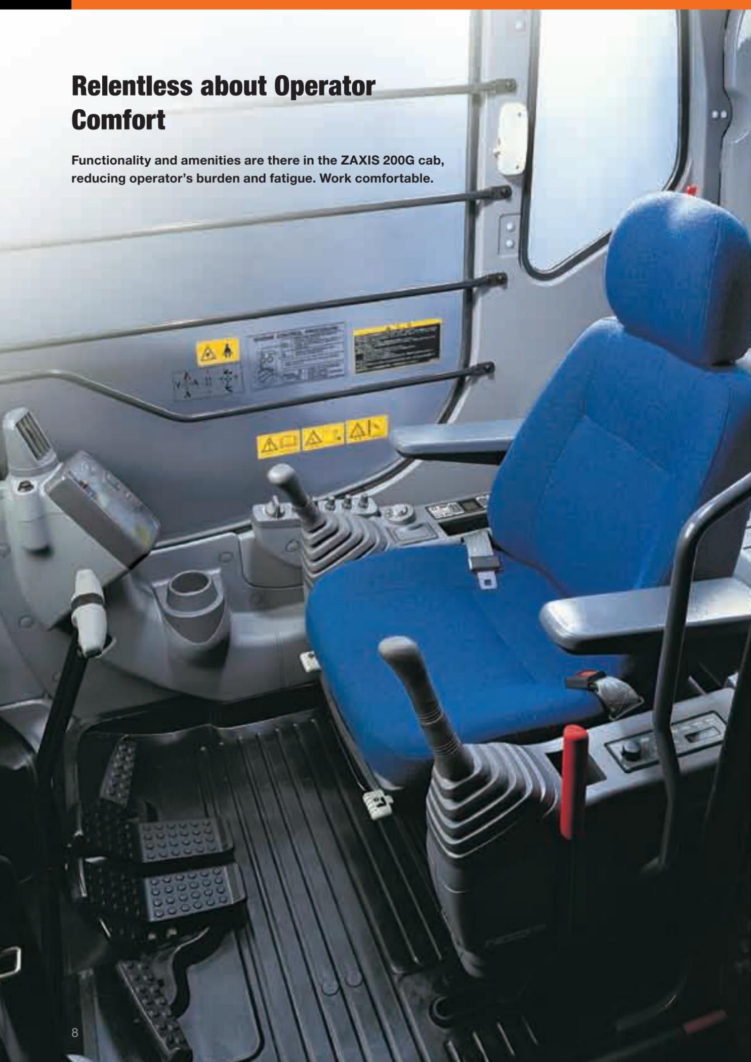
The comfort-designed cloth-covered seat is fitted with a headrest and armrests. The seat can be finely reclined and slid to suit each operator build for comfortable positioning. This allows long-hour operation with less fatigue.
